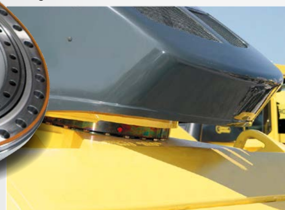
Tandem asphalt vibratory roller with a slewing ring as the steering bearing and high pre-loaded ball slewing rings with special sealing in the split bandage (roller)
