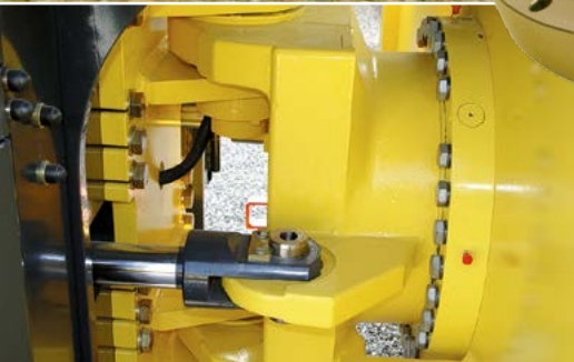
Vibratory rollers such as landfill compactors with surface-coated slewing ring in the knuckle joint
